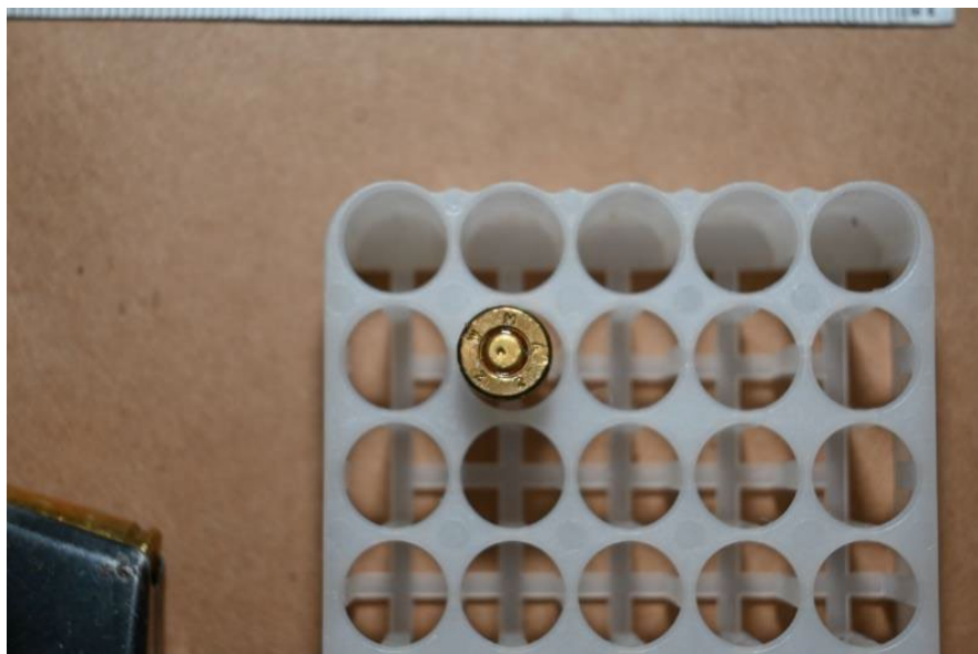
[Light firing pin impression from chambered cartridge]
